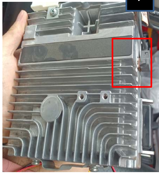
Hier sitzt das LVDS (DISPLAY) Kabel / This is where the LVDS (DISPLAY) cable is located
