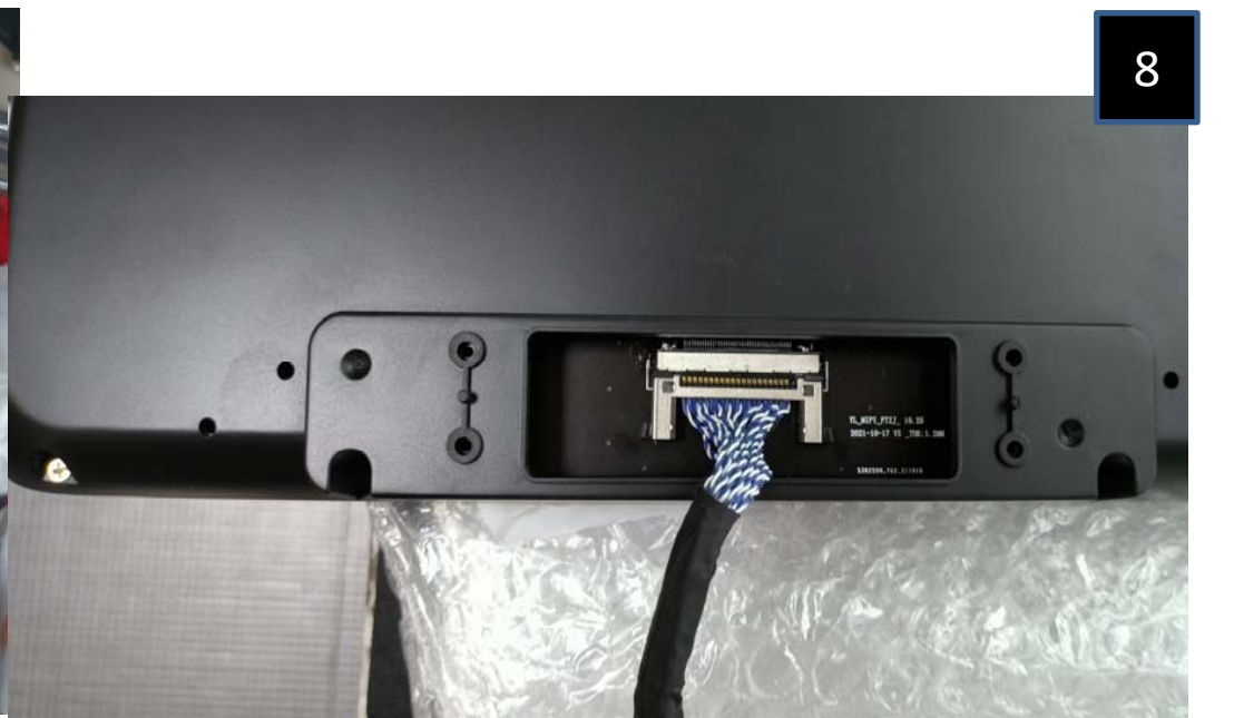
Hier sitzt das LVDS (DISPLAY) Kabel / This is where the LVDS (DISPLAY) cable is located
