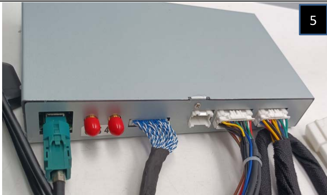
Hier sitzt das LVDS (DISPLAY) Kabel / This is where the LVDS (DISPLAY) cable is located
